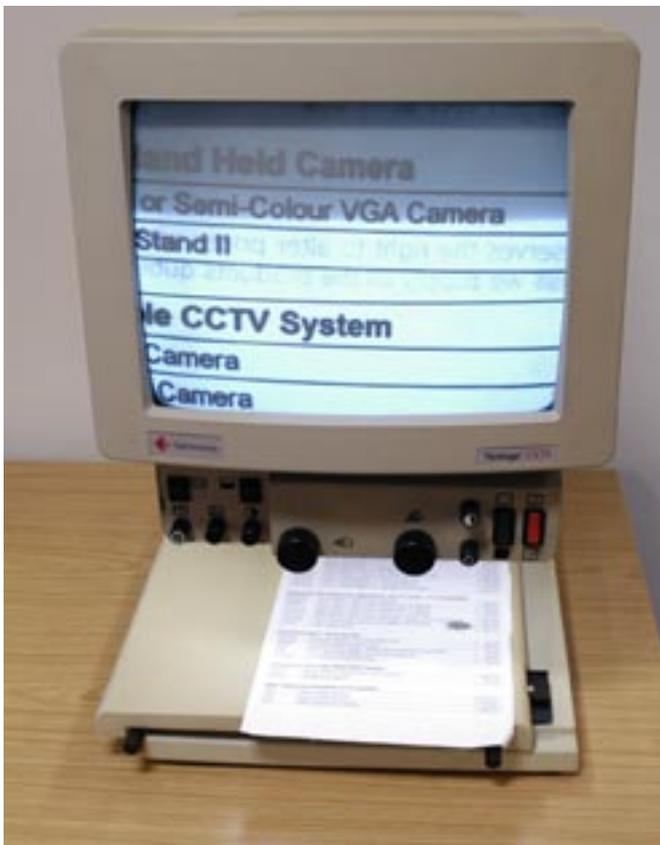
**A early model Telesensory Vantage CCD with X-Y table and line-markers**
