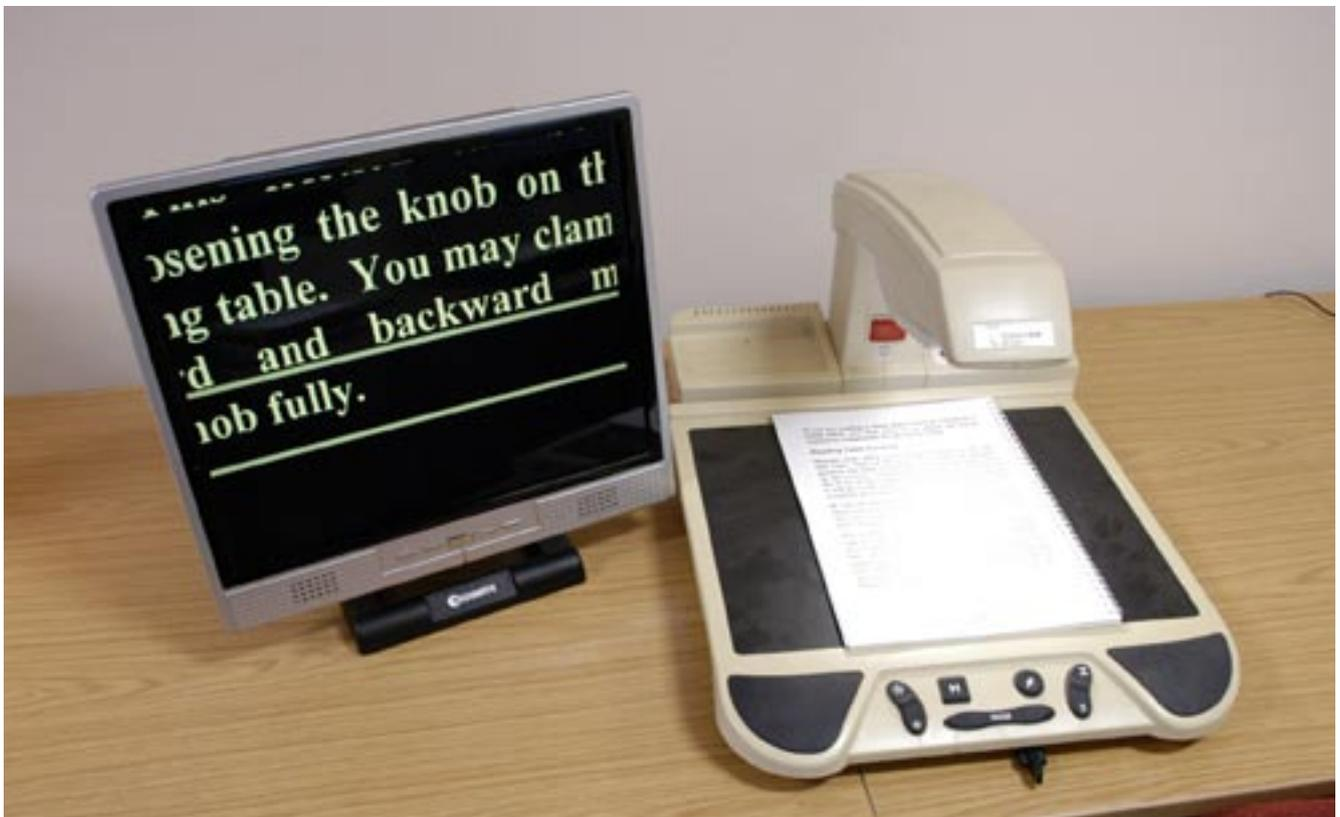
**Optelec Tieman Clearview Bright reading device that can be attached to a computer monitor**
