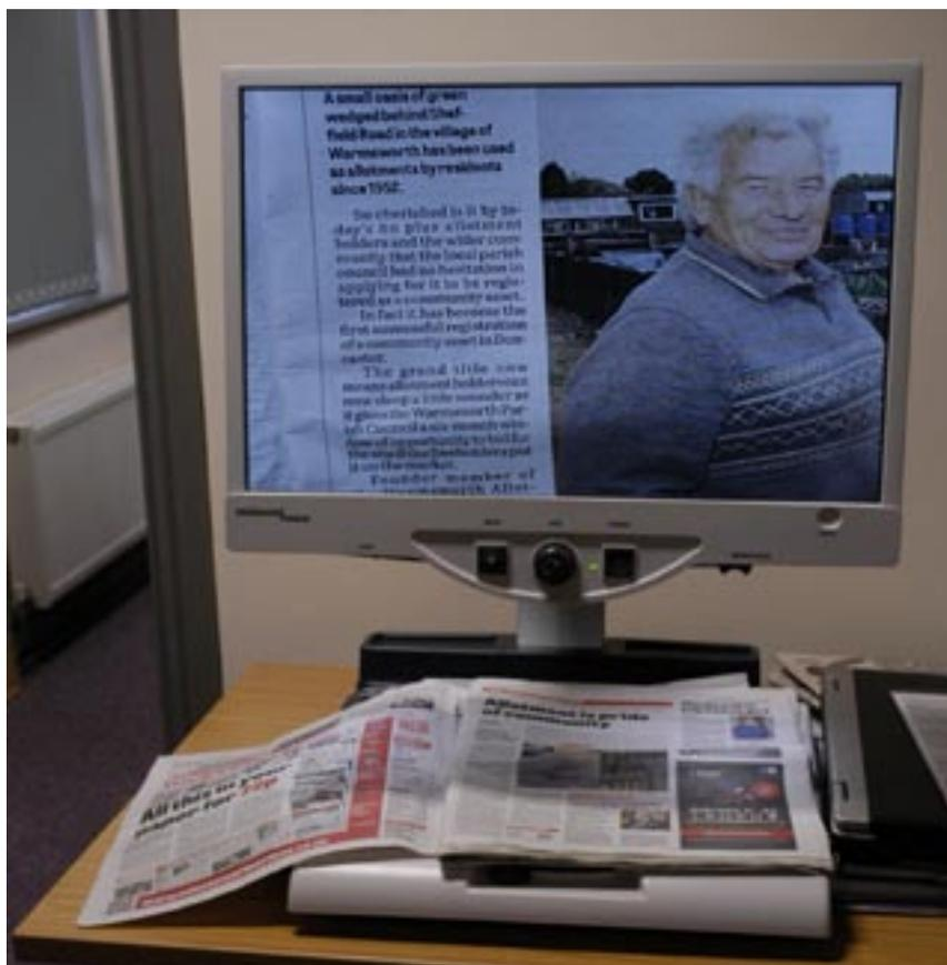
**The Merlin Enhanced Vision optical reader with x-y table, large full colour LCD screen and a range of colour and magnification options.**
